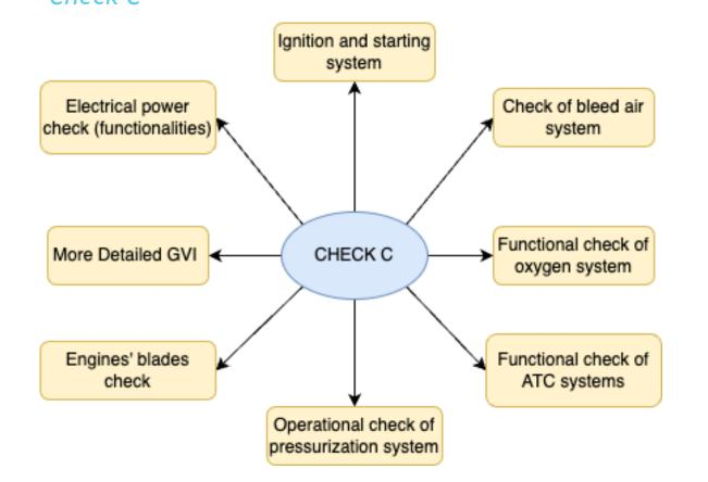
A more detailed inspection increases the likelihood of identifying damaged parts, thus non-functioning, consequently raising the probability of resorting to off-aircraft maintenance!
