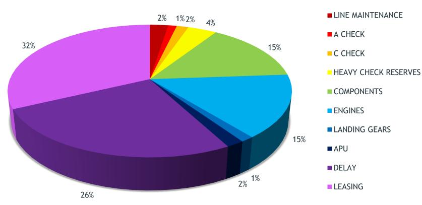
The figure represents, in a pie chart, the percentage breakdown of the total maintenance cost (direct, indirect, and consequential).
