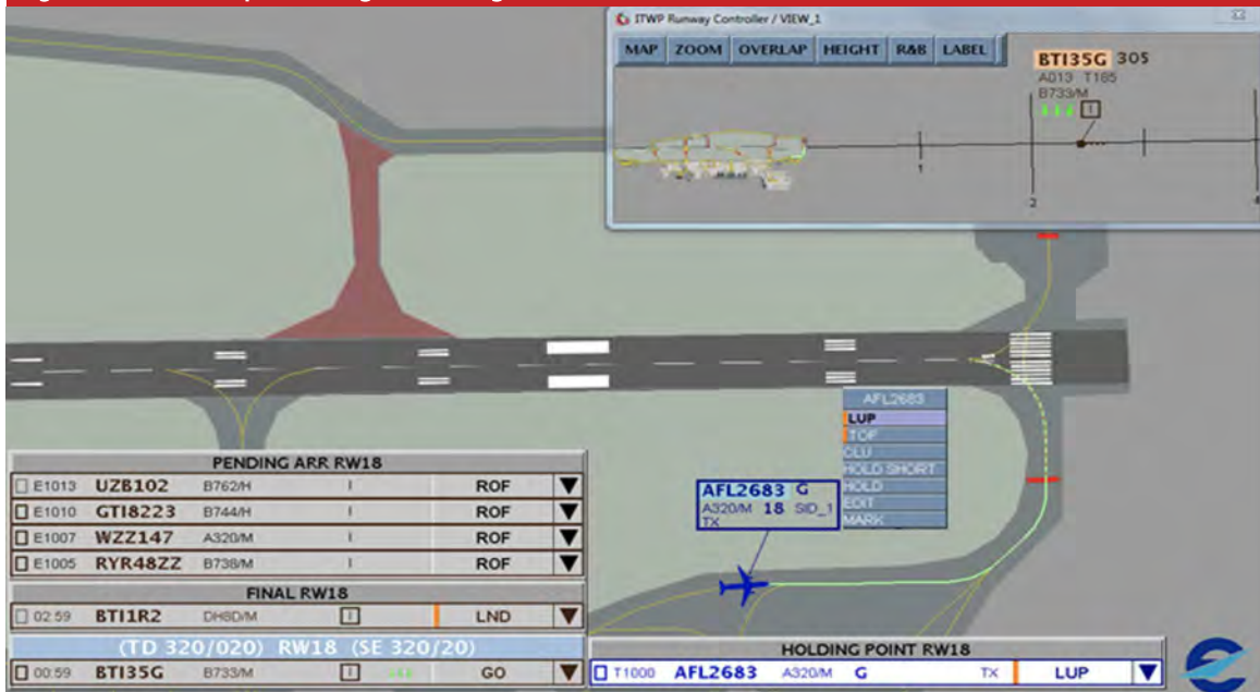
Figure 24. ASMGCS preventing conflicting ATC clearance
