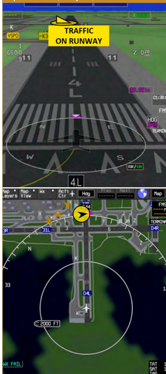
Figure 42. Example of SURF-IA prototype implementation (Honeywell).
